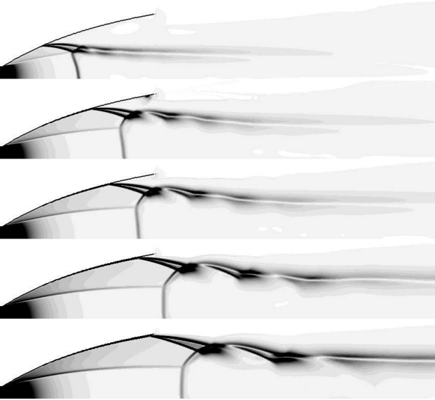
Fig. 18 DLR PAR contour, pseudo-schlieren plots of computational results (from top to bottom) p_c/p_a = 16, 32, 40, 56, and 72 .
