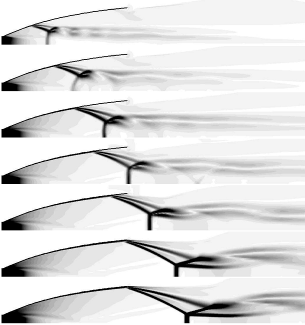
Fig. 9 DLR TIC contour, pseudo-schlieren plots of computational results (from top to bottom) p_c/p_a = 10, 20, 30, 40, 50, 65 , and 75 .
